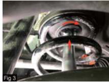
• Insert through the disc and make a half turn to connect the tool and disc
