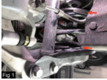
• Place upper and lower discs on spring
