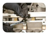
Put on extractor nut turning out broken screw with wrench
